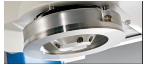
Close-up View of Wall Friction Lid for wall friction test and bulk density test
