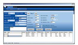
PG Flash allows users to create repeatable custom tests with all of the built-in options on the DV2T plus the addition of multiple program lines (up to 25 steps). Create the program on the PC and download to a USB Flash Drive. Upload the program from the USB Flash Drive to the DV2T.
